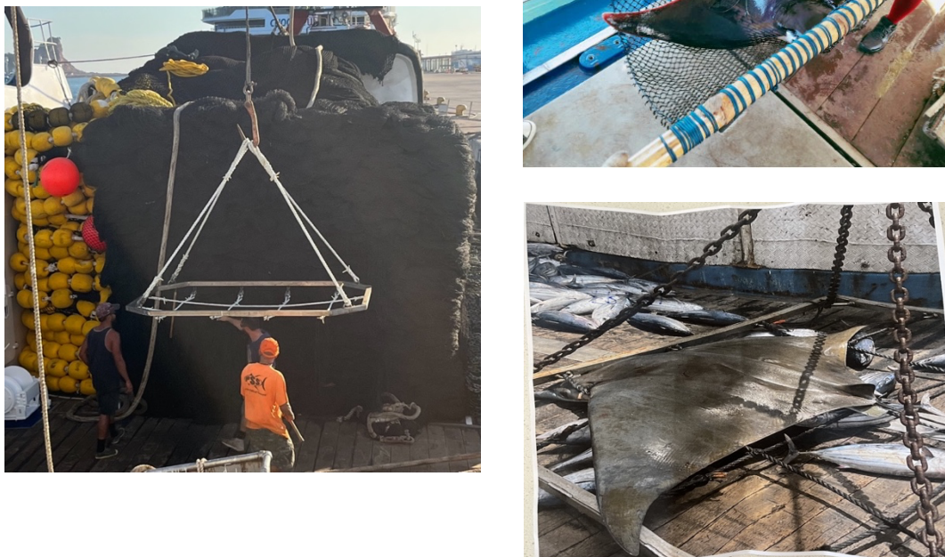
Figure 3. Sorting grid and stretcher used to release Mobulas in the U.S. fleet
